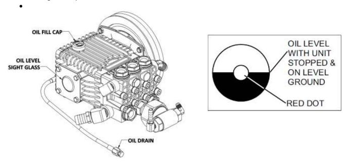
• After the **first 50 hours** of operation, change the crankcase oil Industrial Pump Oil, (Part # 13-030). Change the crankcase oil **every 500 hours** thereafter.
