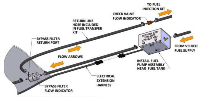
INSTALL BYPASS FILTER NEAR BULKHEAD CONNECTOR
