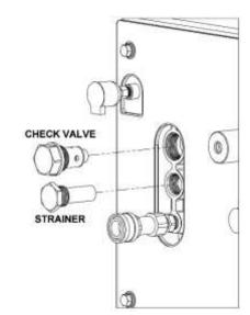
**NOTE:** New o-rings must be installed **anytime** the check valve is removed.
